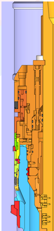
Seal Assembly locked by pressure from the closed ram
